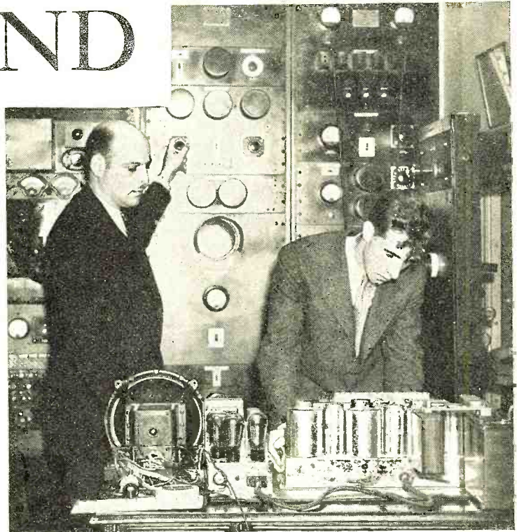
A VIEW OF THE COMBINATION TRANSMITTER Edwin K. Cohan and William B. Lodge operating the new transmitter and a converted Scott receiver used in some of the first tests
