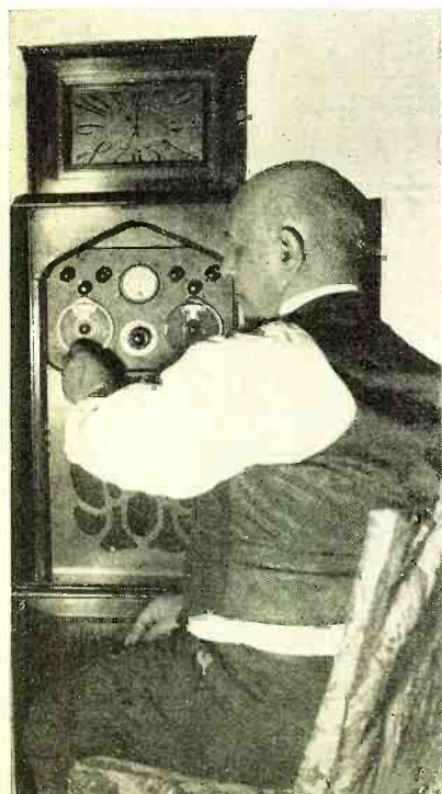
Figure 2. Its tuner unit is built into the same shield as the all-wave receiver tuner, but employs a separate amplifier and power supply
